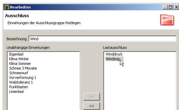
Figure 47: Configuration of action exclusion groups e. g. wind pressure and suction
