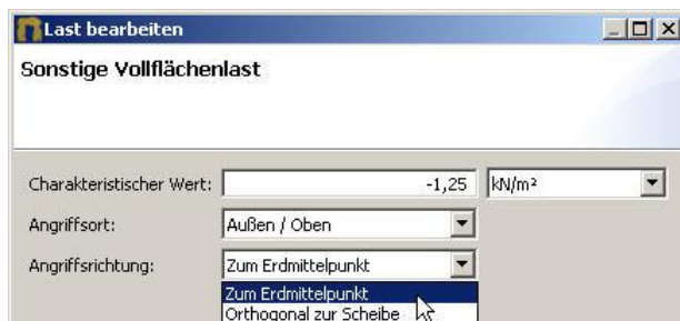
Figure 31: Entering the snow load s_i with a negative sign ("towards the center of the earth")
