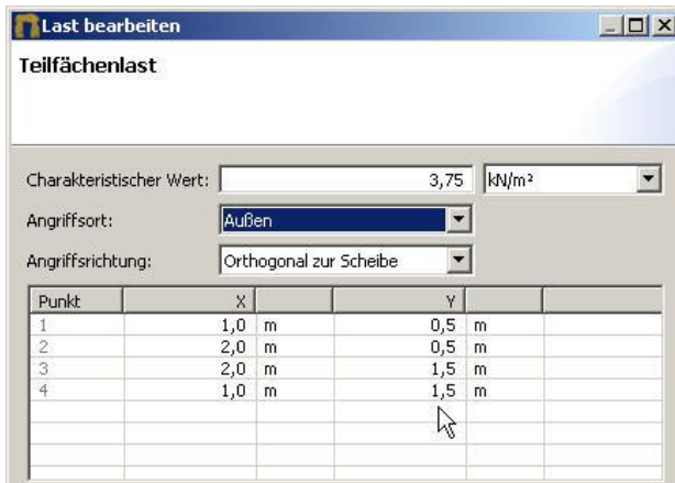
Figure 36: Input of the partial snow load due to the snow removal
