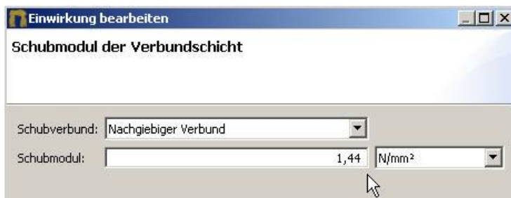
Figure 18: Input of the shear modulus at "partial bond"
